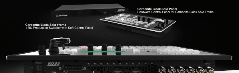
Carbonite Black Solo all-in-one 3G Production Switcher Combined Electronics and Control Panel
